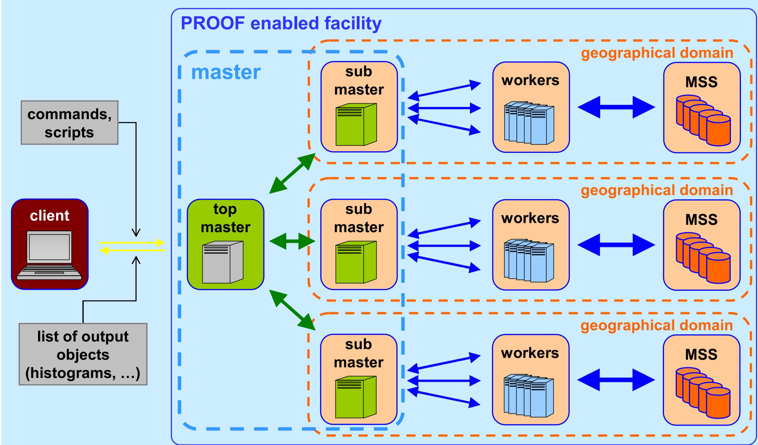
Connection lay-out set up via dedicated daemons in charge of authenticating the clients and spawning the server applications. XROOTD [2] has been instrumented for this purpose.
